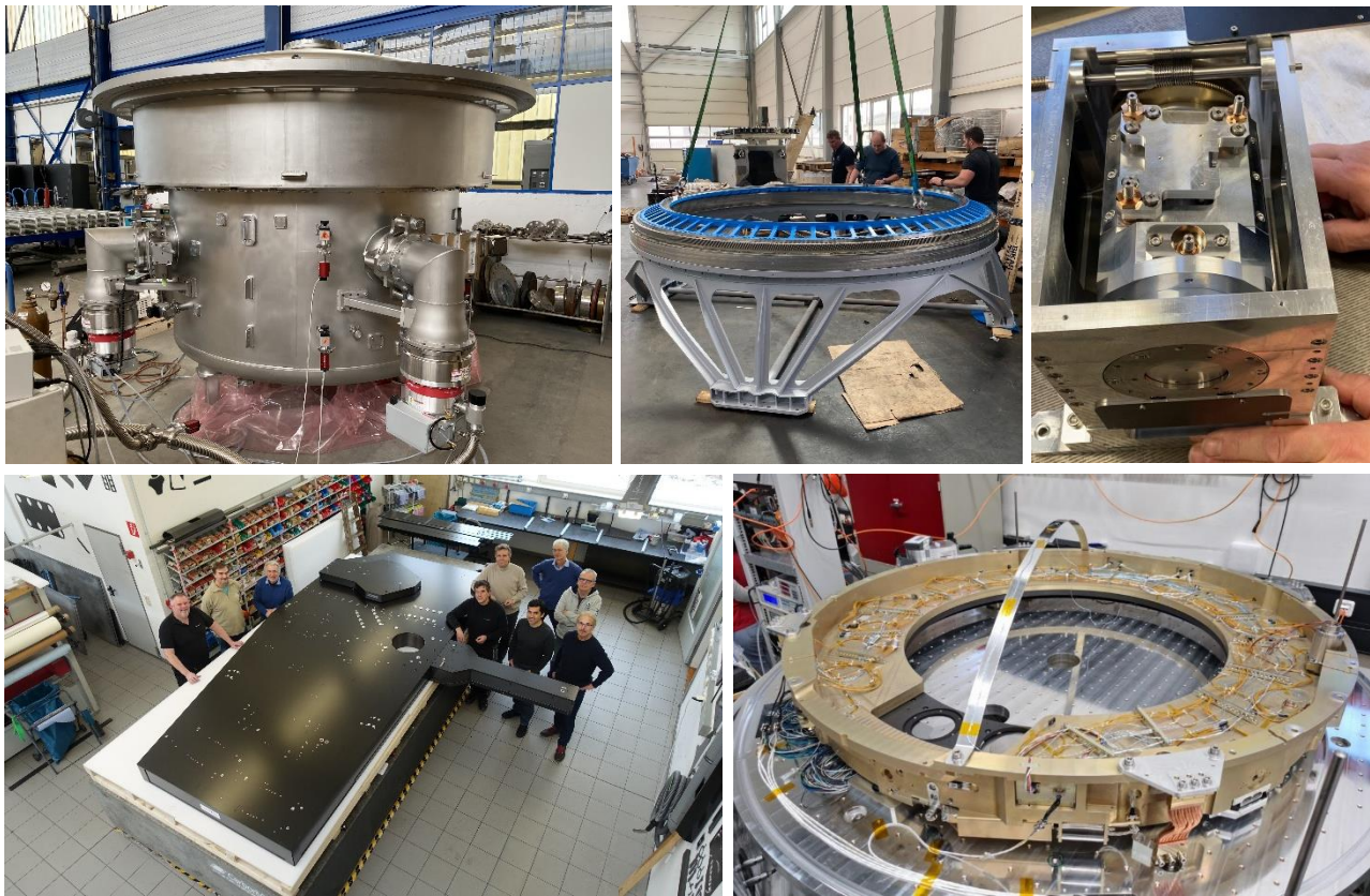
Figure 4: Top left: the MICADO cryostat during (successful) vacuum testing. Top middle: (successful) acceptance testing of the De-Rotator. Top right: The SCAO K-mirror. Bottom left: The MICADO Relay Optics Bench during (successful) acceptance by the MPIA MICADO team. Bottom right: The pupil wheel mechanism being prepared for the (successful) cold sub-system tests.
