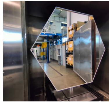
After coating and I/Fs PADs application, one segment performed thermal test
