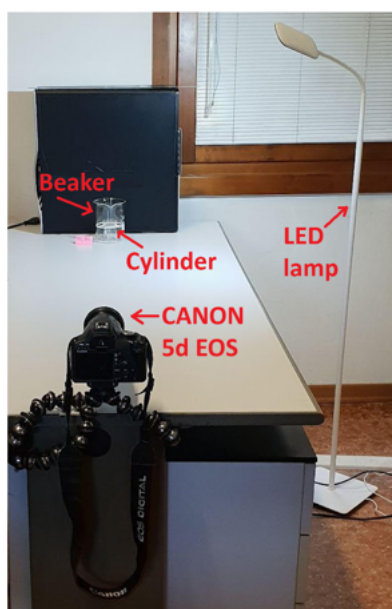
Fig. 3. Experimental set-up employed for the refractive index calculation.
