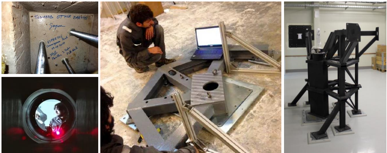
Figure 8: (top left) the central pin at the convergence point was the first hardware piece of ESPRESSO installed at Paranal, on July 3 rd , 2014; (bottom left) the laser tracker pointed in the Coudé Room of UT2; (center) balancer and plates during alignment before gluing; (right) FE structure mounted in the CCL.
