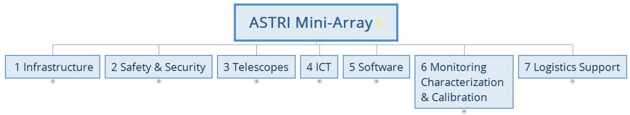
Fig. 3. The ASTRI Mini-Array system decomposition showing the main subsystems.
