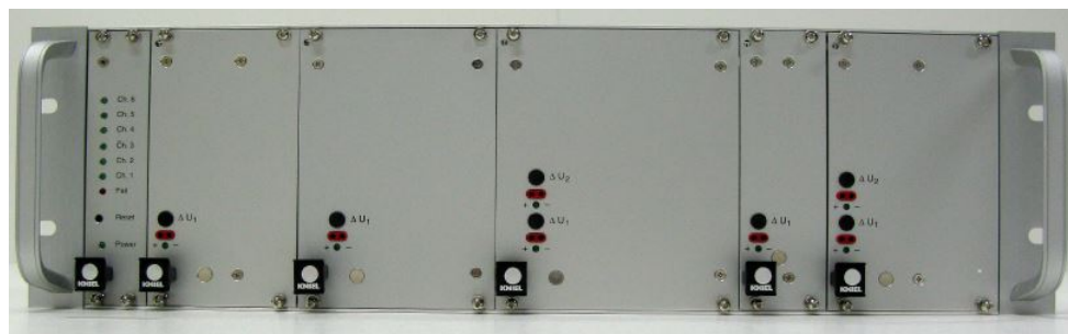
Figure 9. Power supply (front view).
