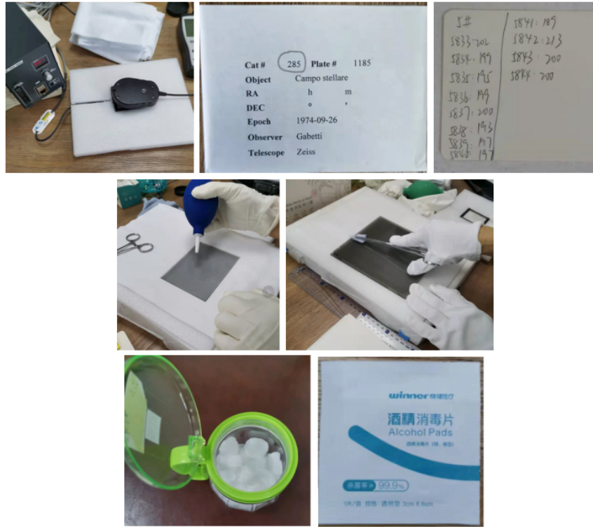
Figure 5: Plate preparation for scanning at SHAO
