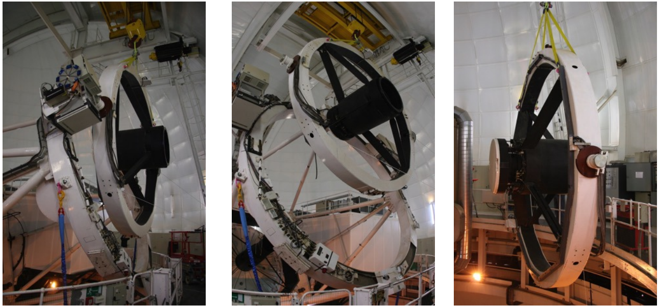
Figure 3: First trial removal of the current top-end ring as an operational test in mid-July 2016.
