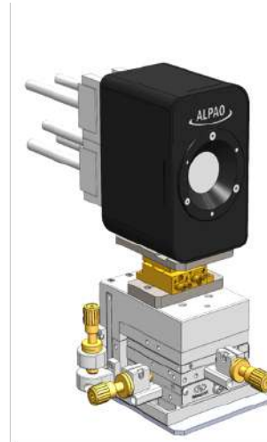
Figure 4-5 A commercial ALPAO High Stability Deformable Mirror on the testbed bench (left) and the CAD model image (right). A pair of DMs are used to simulate the GMT M1 & M2 figure control.
