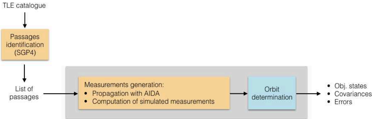
Fig. 7 Architecture of BIRALES simulator.
