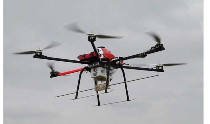
Fig. 1. A micro-UAV equipped with a RF generator and a dipole antenna.
