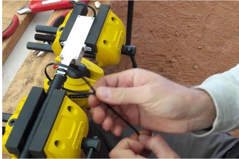
Figure 23: Cable ties tightening.
