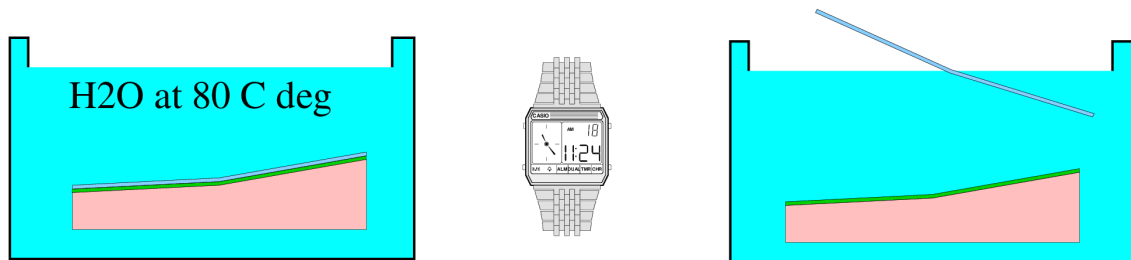
Fig. 9. Ungluing of the substrate from the spacer in hot water.
