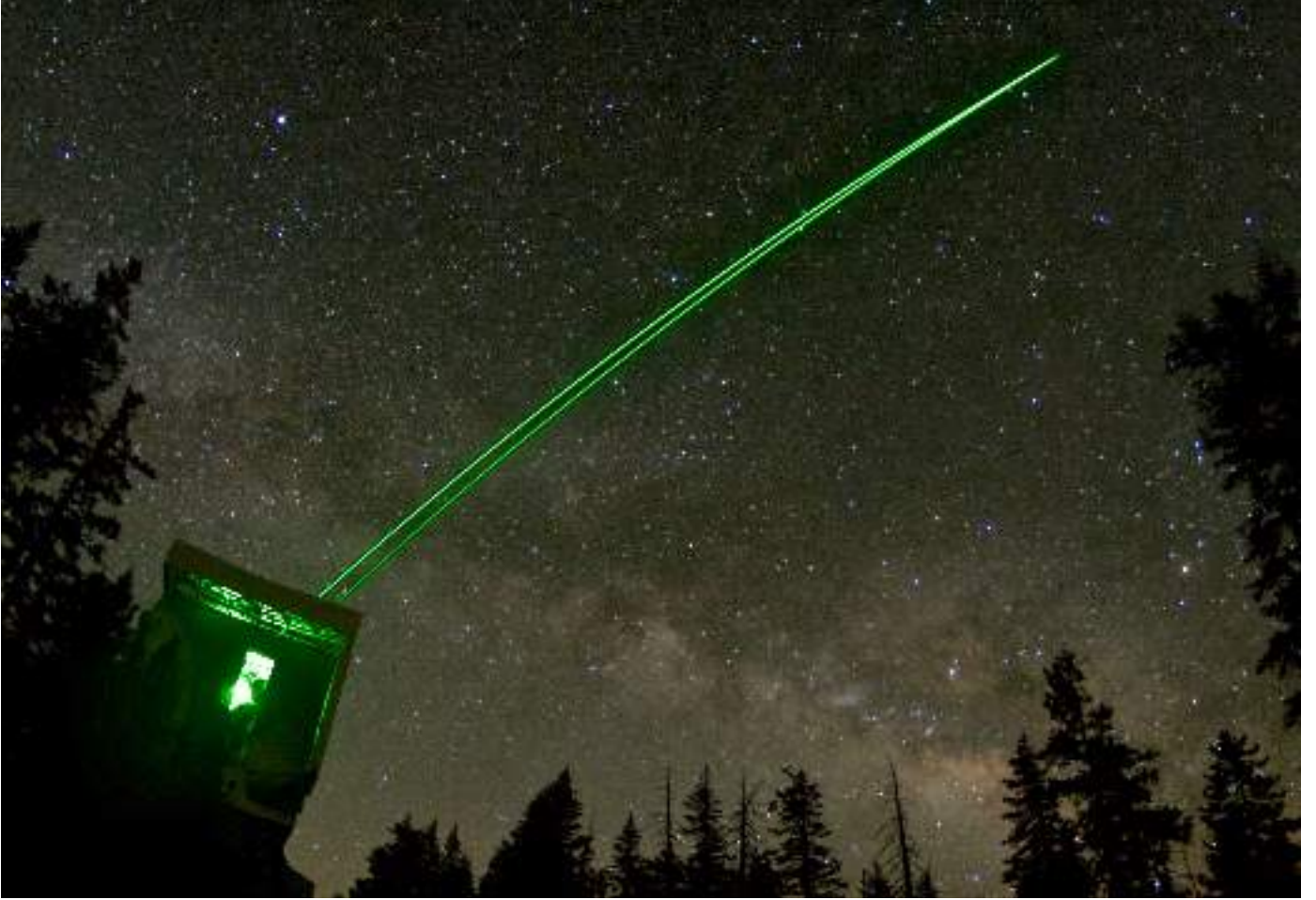
Fig. 1. The ARGOS system propagating a bundle of laser beams on each side of the large binocular telescope. This wide-angle photograph was taken in 2017 with a 25 s exposure time. Each visible green beam in this image consists of three individual laser rays forming the wide-field constellations of guide stars in the atmosphere. The light pulses from the high-power lasers are subject to Rayleigh scattering by air molecules in the Earth’s atmosphere. Having the wavefront sensors gated and adjusted to receive the photons only from a distance of 12 km, a sharp reference beacon constellation is formed. Measuring the wavefronts and correcting the atmospheric ground-layer distortions with the two adaptive secondary mirrors yields a wide-field correction for imaging and spectroscopy.
