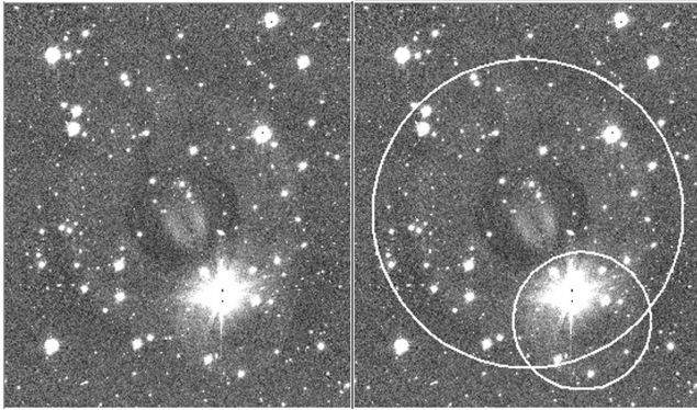
Figure 7. Left: small and large stellar haloes, due to reflection from different pairs of surfaces within the VST. Right: same image, displaying the two types of halo masks demarcated by small and large circles. The reflection halo centroids are offset from the star; relative to the centre of the field of view, the small (large) halo centroids lie inwards (outwards). The bright star in these images has an r magnitude of \sim 10 . The large circle has a radius of 210 arcsec.
