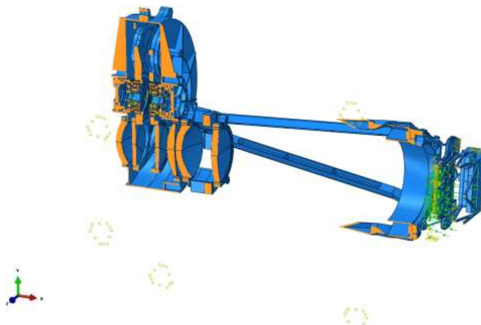
Figure 9-5 All loads applied on steady state analysis
