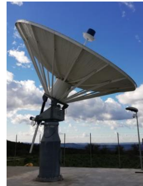
Fig. 2 BIRALES transmitting antenna (TRF).
