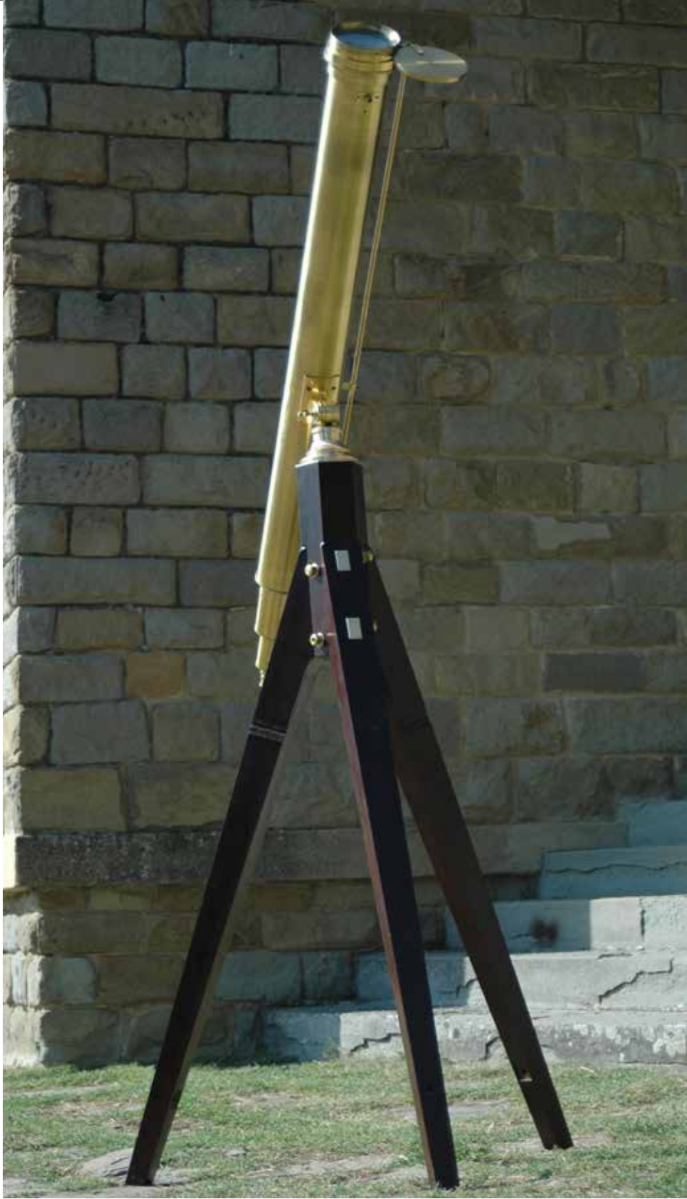
FI. 09. REFRACTING TELESCOPE Steinheil (obiettivo), Munich 1858 brass, wood, glass (objective: 108 mm diameter, 1620 mm focal distance) INAF-Arcetri Astrophysical Observatory, inv. Coll. Scient. e Museali n. 107005001
