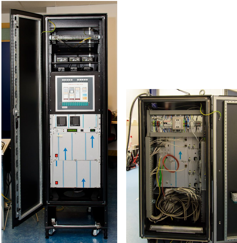
Figure 4 Instrument Main Cabinet on the left and Front End Unit Cabinet #4 on the right, both with double PLC subracks
