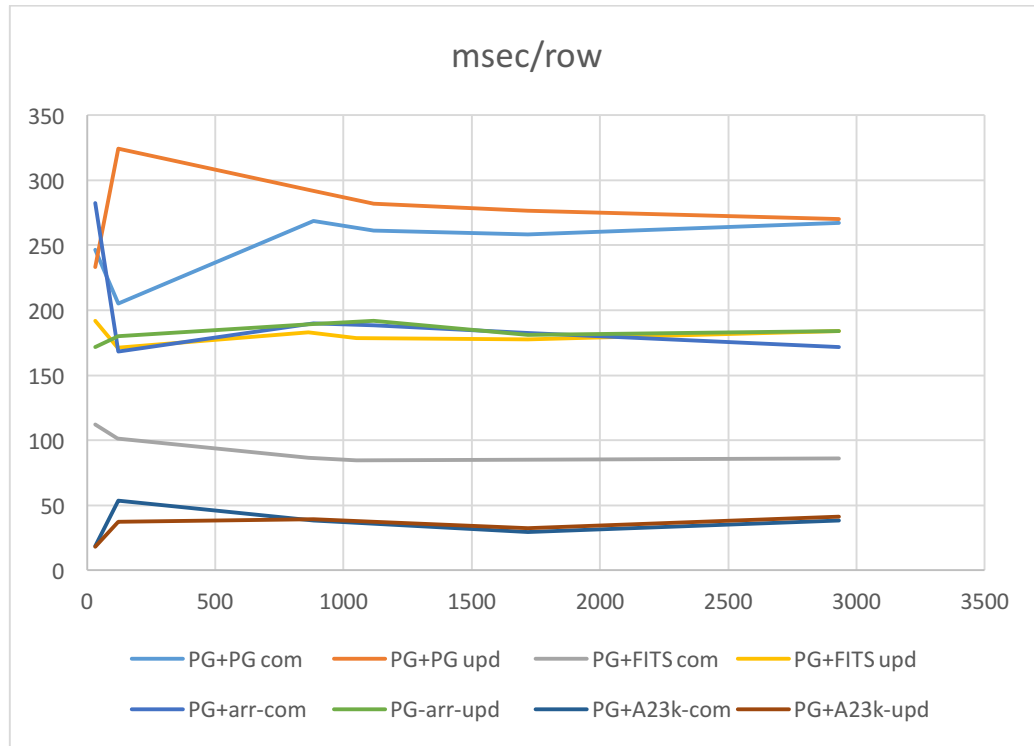
Figure 4. Mean time spent calculating the S-index for the sets of stars as in Table 3. Four methods are plotted, each with its values for just computing (com) and those also for updating (upd) the header tables with the new values. PG+PG: PostgreSQL with spectra stored as csv text; PG+FITS: spectra values are accessed opening the corresponding FITS file; PG+arr: spectra stored as SQL array; PG-A23k: spectra stored as SQL array but only the first 23k values (of 300k) are retrieved by the query.
