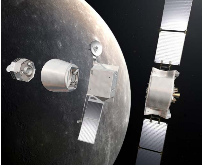
Figure 1.5. Artist's impression of BepiColombo spacecraft cruise modules. From left to right: Mercury Magnetospheric Orbiter, Sun Shield, Mercury Planetary Orbiter, Transfer Module (courtesy of ESA/AOES Medialab).
