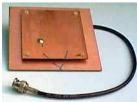
Figure 2.5: Example of a patch antenna.
