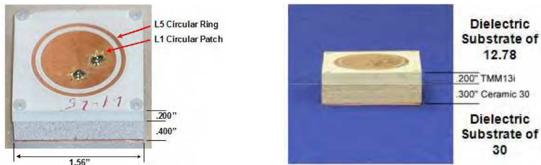
Figure 2.10: Top and Side Views of Dual-Band Co-Planar Patch Antenna.
