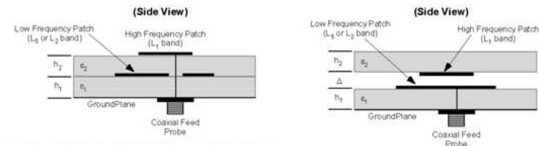
Figure 2.8: Dual-band Stack patch antennas.
