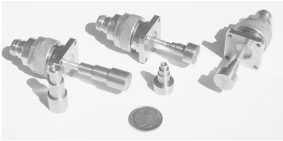
Fig. 3. Photograph of the probes. The input probe and assembled input probe-connector combination are shown on the left. The two assembled output probe-connector combinations (and one unassembled output probe) are shown in the center-right. The 7/16-type to N-type connector transitions attached to the 7/16 connectors were used for test of the devices.
