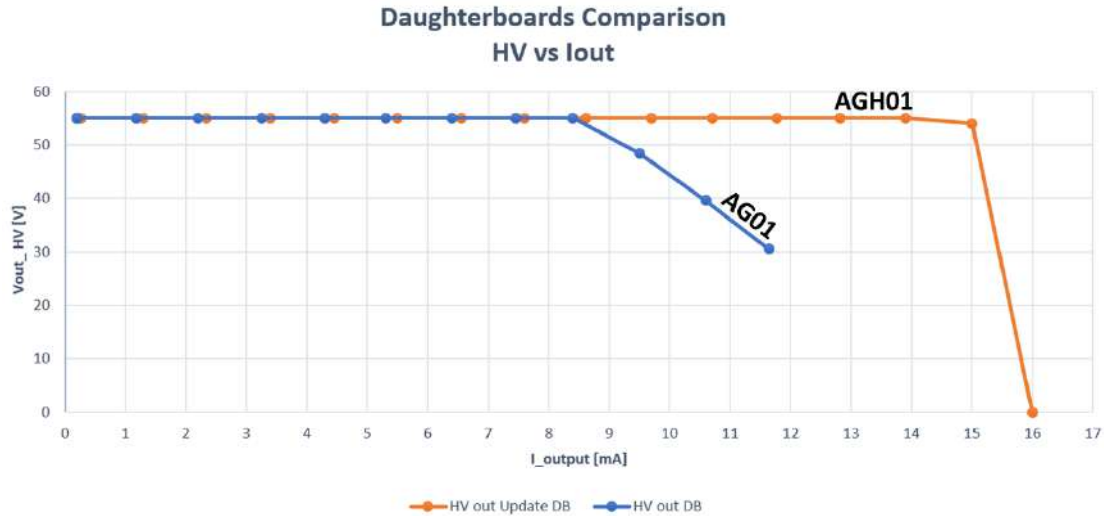
Figure 10. Comparison between the output currents of the daughterboard before and after the modifications. The updated daughterboard, equipped with the AGH01 provides more current than the one with the AG01 DC-DC converter. The current provided to the SiPM detectors is almost doubled, actually extending the observation time thanks the possibility to work with a higher level of NSB.
