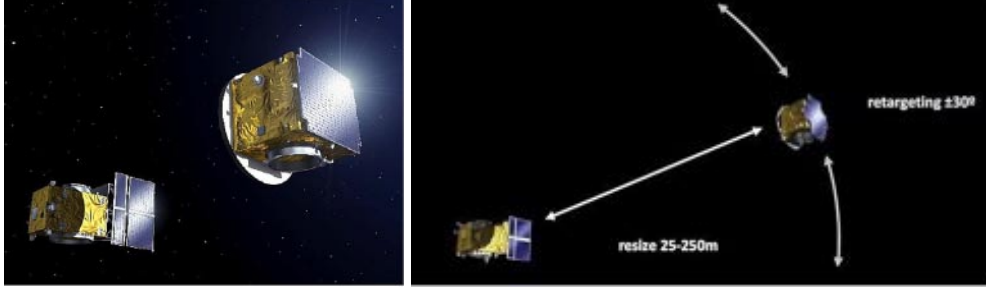
Fig. 1. – Positioning of the two spacecraft during observations (not in scale) and FF demonstration maneuvers performed with reference to the Sun direction.
