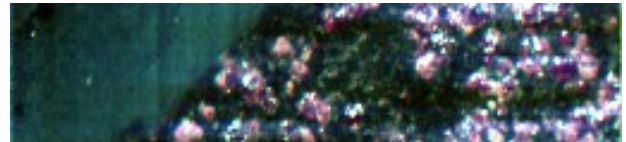
Fig.1. RGB image acquired with SPIM on the thin section (R:0.70 \mu\text{m} , G:0.53 \mu\text{m} , B:0.44 \mu\text{m} ).
