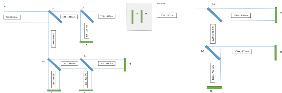
(a) Schematic division of the visible arm. (b) Schematic division of the infrared arm.
