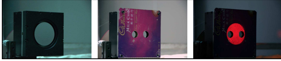
Figure 4. On the left the expected geometry of the four-pupils image and on the right a picture of what was actually obtained.
