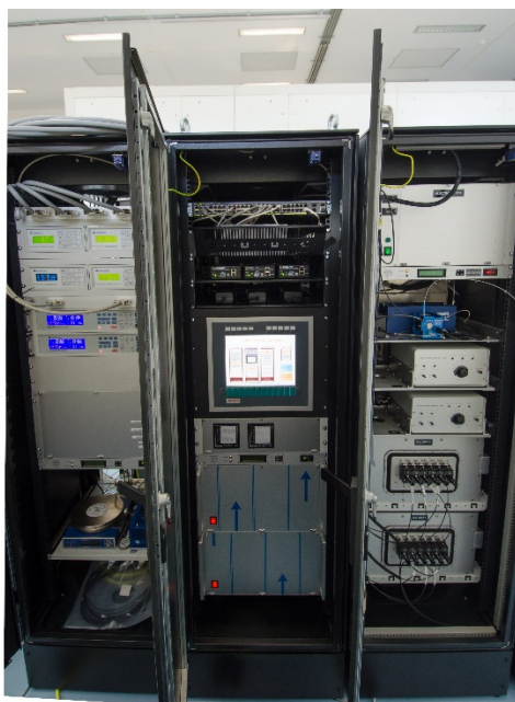
Figure 3: Thermal control cabinet (left), Instrument main cabinet (center), Calibration unit cabinet (right) were tested with all the other subsystems, satisfying the requirements.
