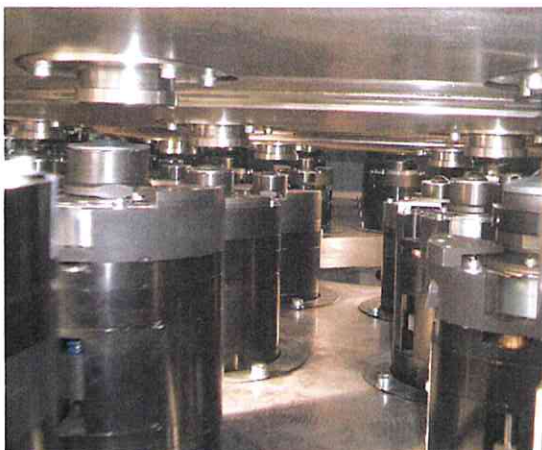
Fig. 12 – Primary mirror handling procedure (2/4): lowering the mirror on the axial supports.
