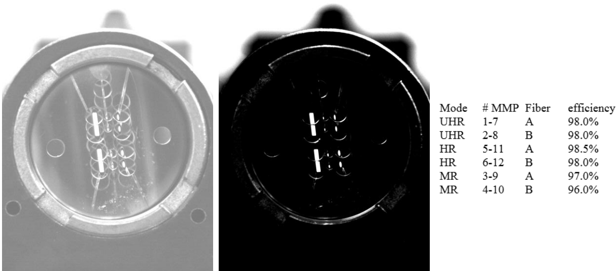
Figure 8: MMP#3 during integration in the APSU. Enhanced brightness image to show the mechanical references in the mounting (left); virtual slits on the MMP plane: four images for each observation mode, made by star and sky fibers, sliced in two (center); transmission efficiency of the single fibers (right).
