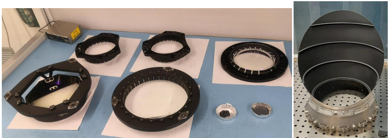
Figure 2. OMGs: mounting delivered by UBE and integrated with lenses at Leonardo Company on the left. The Baffle Assembly after painting delivered by TAS-I on the right.
