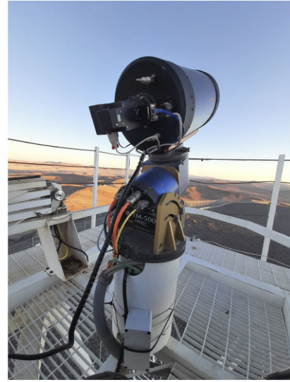
Figure 2. ESO MASS-DIMM located at Cerro Paranal, site of the VLT in Chile. The instrument is placed on top of a 7-m high tower. Credit: Angel Otarola, ESO.
