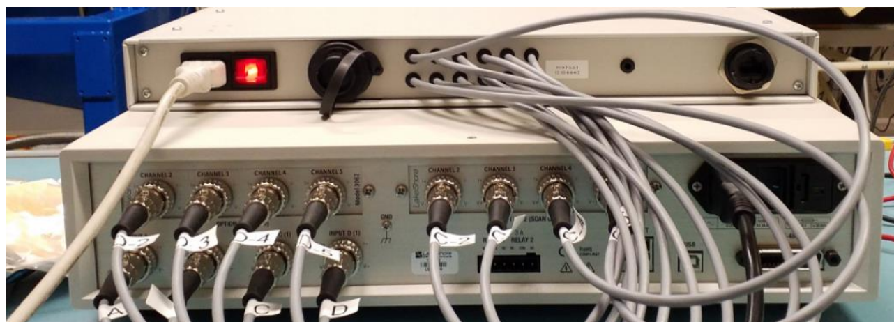
Figure 25 Harness from Multiplexer to Lakeshore. Labels are reported in §0
