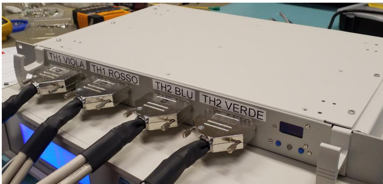
Figure 26 Multiplexer: cables labelling. Colours and names are the same reported in §0
