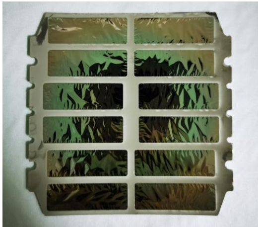
Figure 8 Left: Demonstration model of the HERMES-TP/SP filter manufactured by IHEP (Beijing). Right: Soft-X/UV/O/IR transmission of the optical filter estimated with different thickness of polyimide (1 \mu\text{m} and 2 \mu\text{m} ) and different total thickness of Al coating (200 nm and 300 nm) deposited on one or two sides of the polyimide substrate
