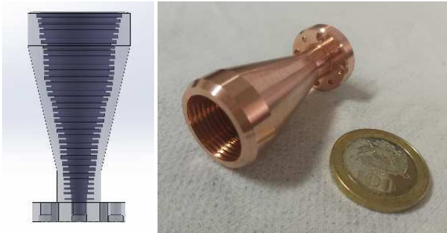
Fig. 9. Computer model of UdC horn (left) and picture of the final copper version (right). A 100 Chilean peso (CLP) coin is shown for scale (23.5 mm).
