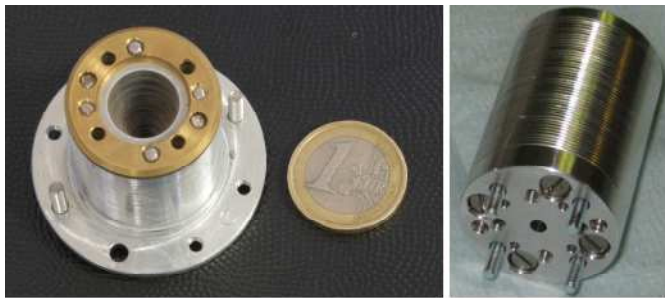
Fig. 11. Mouth (left) and waveguide interface end (right) of the platelet feedhorn produced by INAF. A 1 euro coin is shown in the left panel for scale (23.25 mm). The total length of the feedhorn is 41.4 mm, and the outer diameter is 12.92 mm.
