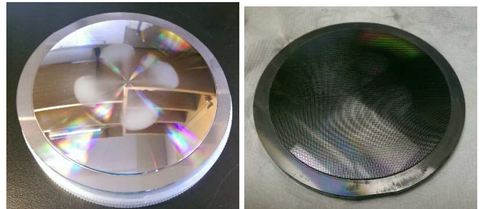
Fig. 7. Photos of the silicon lens prototype. Left panel: lens blank, which was produced by Nu-Tek Precision Optics using a CNC lathe. Right panel: lens after application of an AR surface layer manufactured using a 5-axis dicing saw. The outer diameter of the lens, including the outer ring used for mounting, is approximately 11 cm.
