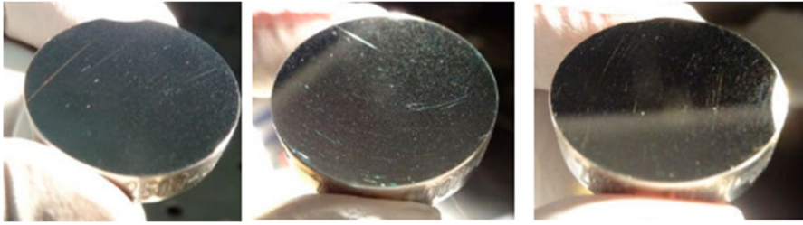
Fig. 13 Representative pictures of one of the aluminum samples before coating (left), immediately after the coating (middle) and after the tests (right)
