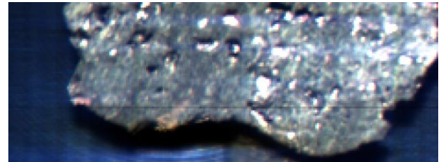
Fig.1. RGB image acquired with SPIM on the meteorite fragment ( R:0.70\text{ }\mu\text{m} , G:0.53\text{ }\mu\text{m} , B:0.44\text{ }\mu\text{m} ).
