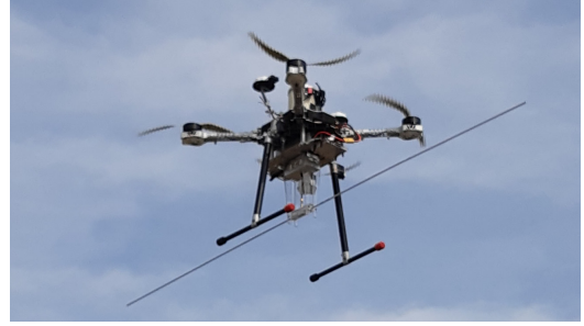
Fig. 3. The UAV-mounted dipole hovering during the measurement.
