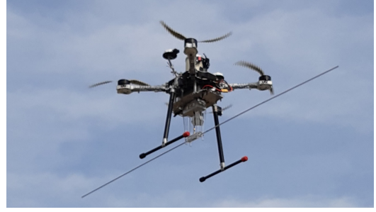
Fig. 3. The UAV-mounted dipole hovering during the measurement.
