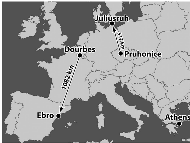
Figure 3. DPS4 observatories and the Digisonde-to-Digisonde skymap links DB → EB and PQ → JR that operated during the case study. The Athens DPS4D, the fifth station of the network, contributed to this event with electron density profile data (see Table 1). DB = Dourbes; EB = Ebro; PQ = Pruhonice; JR = Juliusruh.
