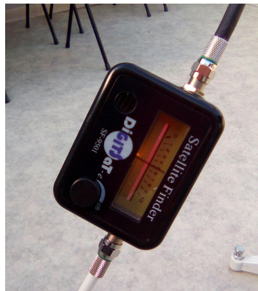
Itty bitty telescope Satellite finder used as receiver
