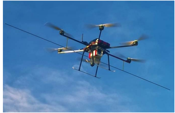
Figure 1: The micro-UAV equipped with RF transmitter, dipole antenna and GNSS system.
