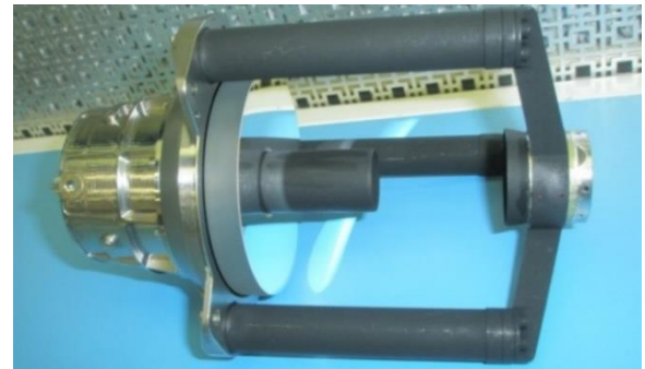
Figure 2: HRIC manufactured optics mounted with internal baffles, mechanical structure (dark grey arms) and corrector holder (light grey cylinder on the left).
