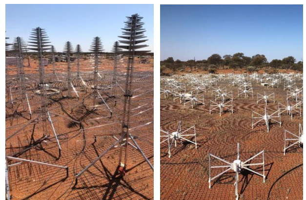
Figure 2. The AAVS1.5 SKALA4.1-AL antennas (left) and the EDA2 bow-tie dipoles (right).
