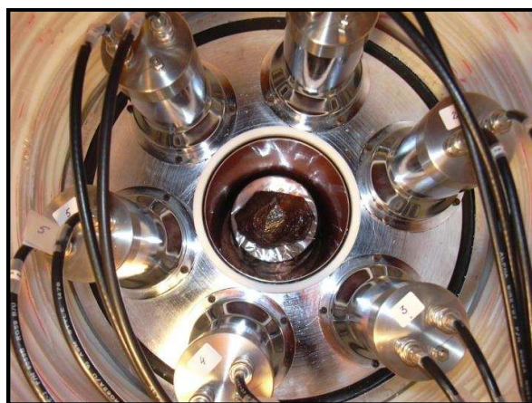
Figure 4 – A detail of the detector of the Monte dei Cappuccini laboratories in Torino.
