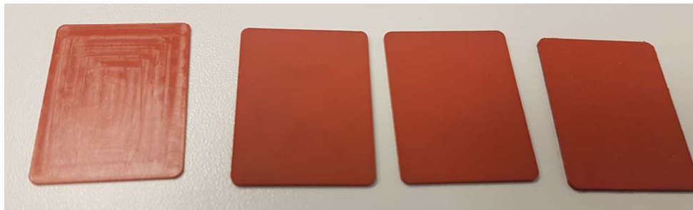
Figure 3. RTV pads prototype samples
