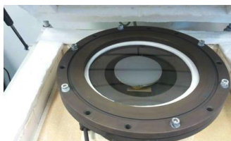
Fig. 8. The setup for the slumping of Eagle glasses on \text{Si}_3\text{N}_4 sample mould: the glass was cut to circular shape with diameter suitable for the application of pressure.
