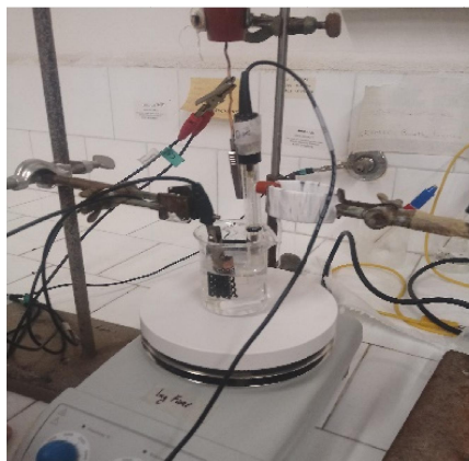
Figure 5 – Experimental setup used for bismuth electroplating.
