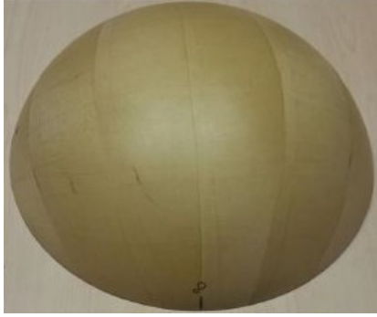
Figure 4. 1mm thick vacuum window developed by NRC (image credited by NRC).
