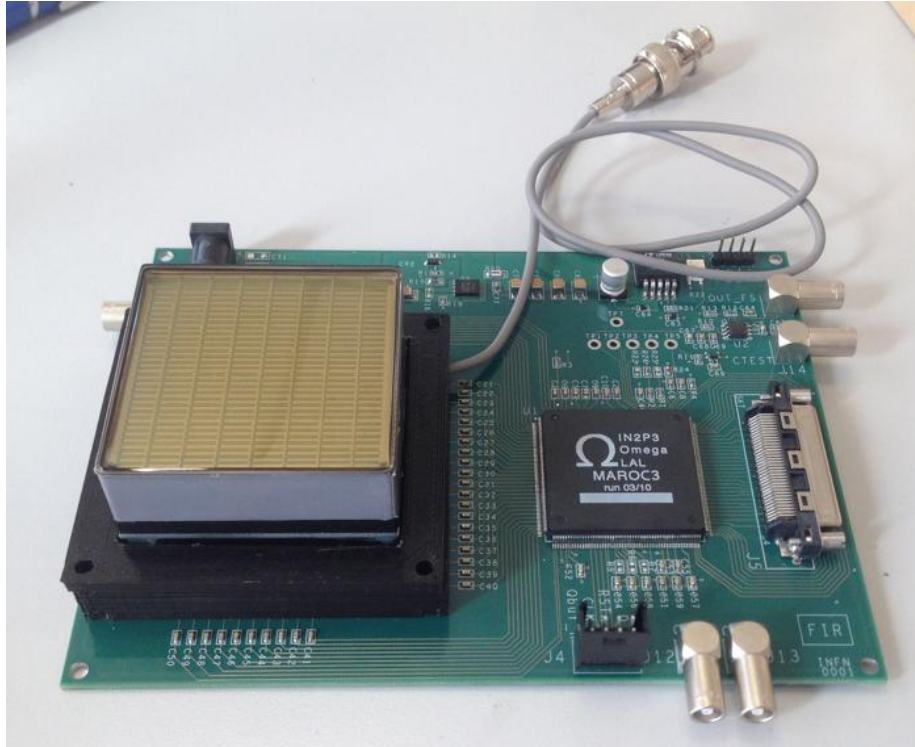
Figure 5: A FE board equipped with a Hamamatsu H8500 64 channels PSPM.
